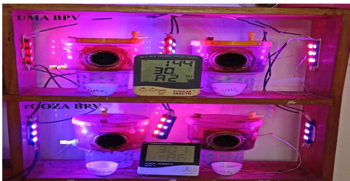
**Fig. 1** Hygro-clocks direct powering ability of the rGOZA and UMA BPVs
